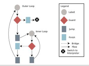
Figure 2. A trace tree constructed by e.g. PyPy's tracing interpreter. It shows a doubly nested loop.
