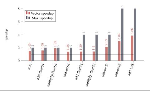
Figure 4. Speedup of the vectorized trace loops. Horizontal line is the baseline for the calculated speedup values ( $speedup = \frac{scalar}{vector}$ ).
