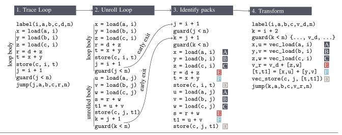
**Figure 3.** Vectorization example. Calculates sum(c) and c[:] = a[:] + b[:]. [a,b] denotes a vector with two elements. Variables that are prefixed with  $v_{-}$  denote vector variables. Vector addition is simply written as  $v_{-}a + [c,d]$ . Step three covers PRE-PARE,BUILDDEPENDENCYGRAPH, INITPAIRS and EXTEND. Step 4. handles COMBINE and SCHEDULE.
