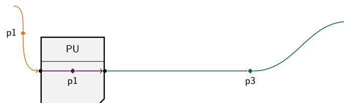
Figure 9: Example of the simple data path from Figure 5 extended by a parallel instruction.
